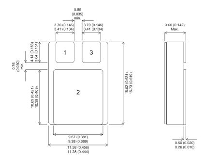
Bipolar NPN Device in a Hermetically sealed Ceramic Surface Mount Package for High
